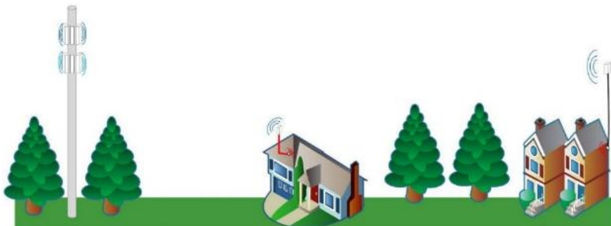
Figure 15: Example Fixed Wireless Network with Antennas on a Monopole and Customer Premises
